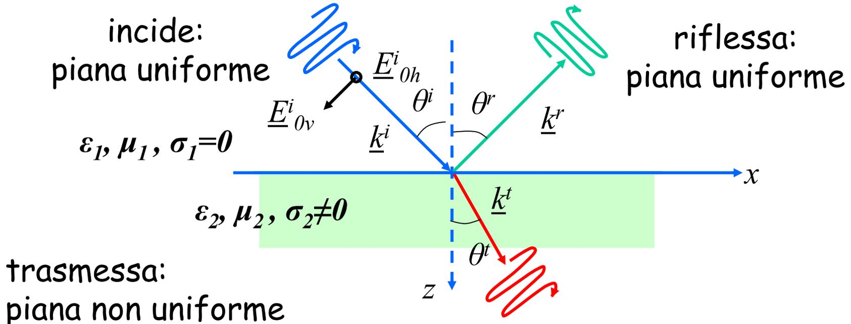
$$\underline{k}^t = \underline{\beta}^t - j\underline{\alpha}^t \Rightarrow \beta_x^t \neq 0; \quad \underline{\alpha}^t = \alpha^t \underline{z}_0$$
