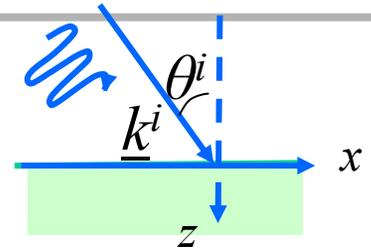
$$\underline{z}_0 \times \left[ \underline{E}_0^t e^{-j(k_x^t x + k_y^t y)} - \left( \underline{E}_0^i e^{-j(k_x^i x)} + \underline{E}_0^r e^{-j(k_x^r x + k_y^r y)} \right) \right] = 0$$
