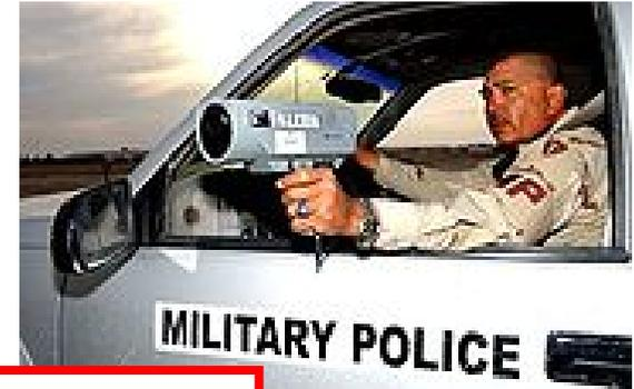
$$f_D = \pm \frac{2f}{c} \underline{V} \cdot \underline{r}_0 = \pm \frac{2 \cdot 24 \cdot 10^9}{3 \cdot 10^8} \cdot 60 = 9600 \text{ Hz} = 9.6 \text{ kHz}$$
