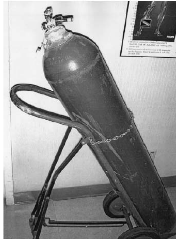
Figure 2. The size “H” oxygen cylinder after the regulator was sheared off. Note the scrapes on the cylinder and the bent beam on the cart.
