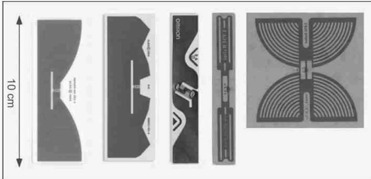
Figure 7.24: Commercial Broadband Structures, Approximately to Scale. (From left: Alien Technology (2), Omron, Rafsec (2)).
