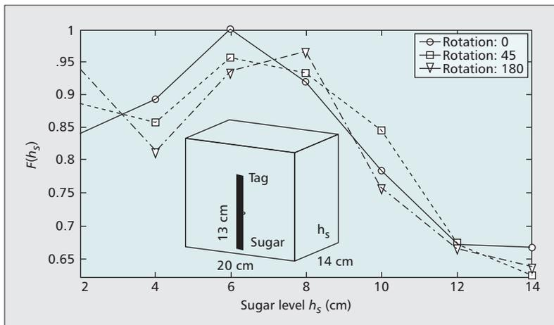
**Figure 3.** Sensing the level of powder (sugar) material by analog, self-sensing modality.
