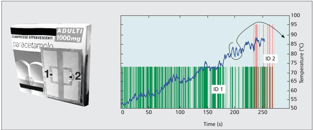
**Figure 4.** Detection of thermal threshold crossing of drugs by a two-port RFID grid used in digital mode.
