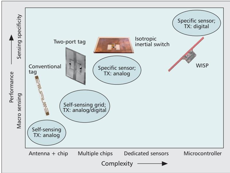
**Figure 2.** Possible classification of passive sensing RFIDs according to the sensing mechanism (self-sensing or by a specific sensor) and data transmission (TX) modality (analog or digital encoding).
