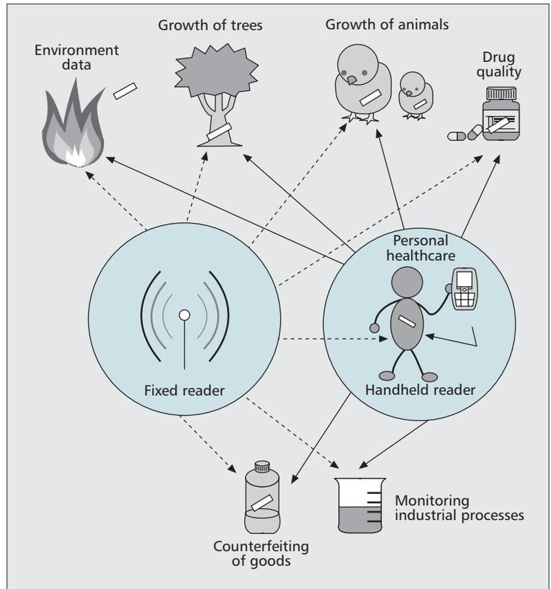
Figure 1. Sensing of Things and humans by fixed and handheld RFID readers.
