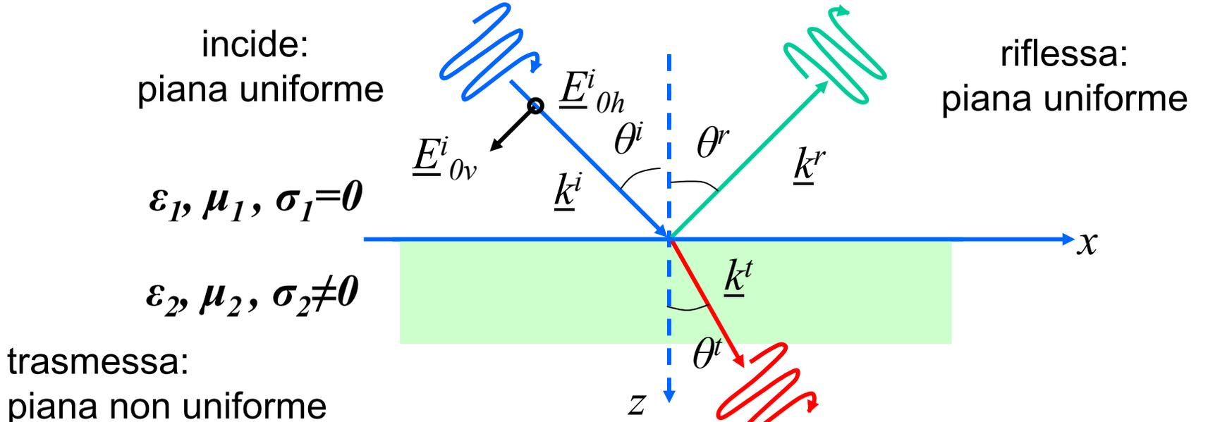
$$\underline{k}^t = \underline{\beta}^t - j\underline{\alpha}^t \Rightarrow \beta_x^t \neq 0; \quad \underline{\alpha}^t = \alpha^t \underline{z}_0$$
