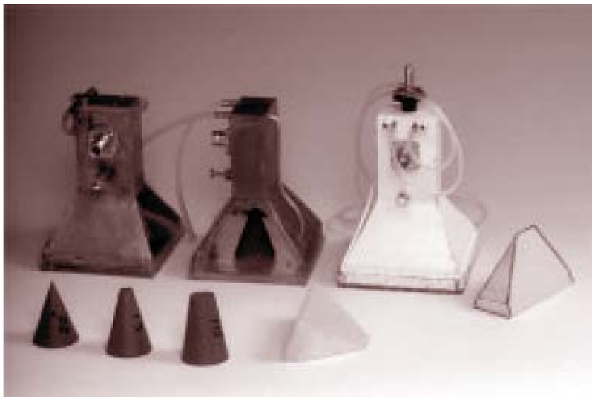
Fig. 1. Various applicators. (left) LA with the two diverging walls of the horn antenna parallel to the electric field made of lucite. (center) LCA similar to the LA with a PVC cone inserted in the center of the antenna. (right) CA made totally of metal.
