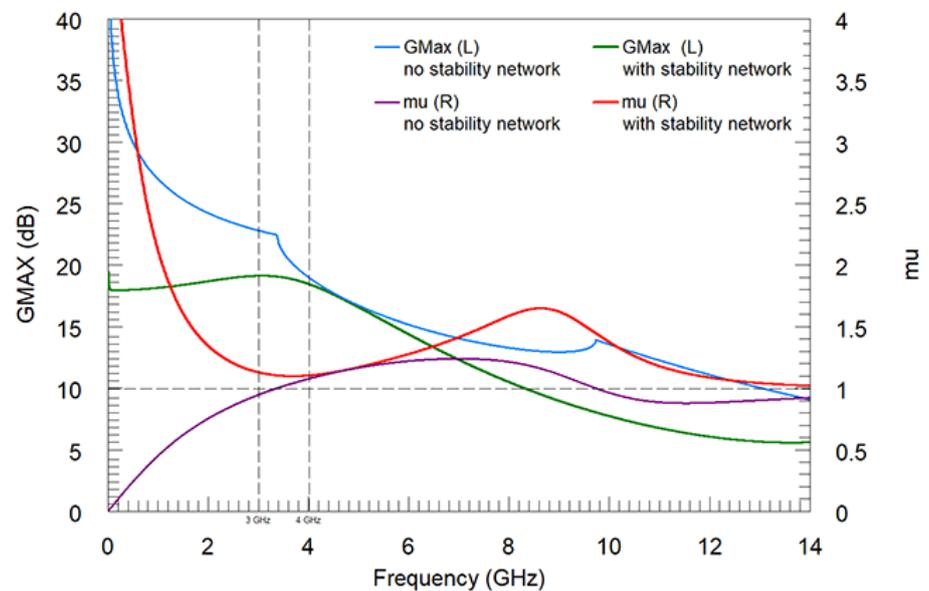
**Figure 3.** Effect of the stability network on maximum available gain ( $G_{Max}$ ) and geometric stability factor ( $\mu$ ).
