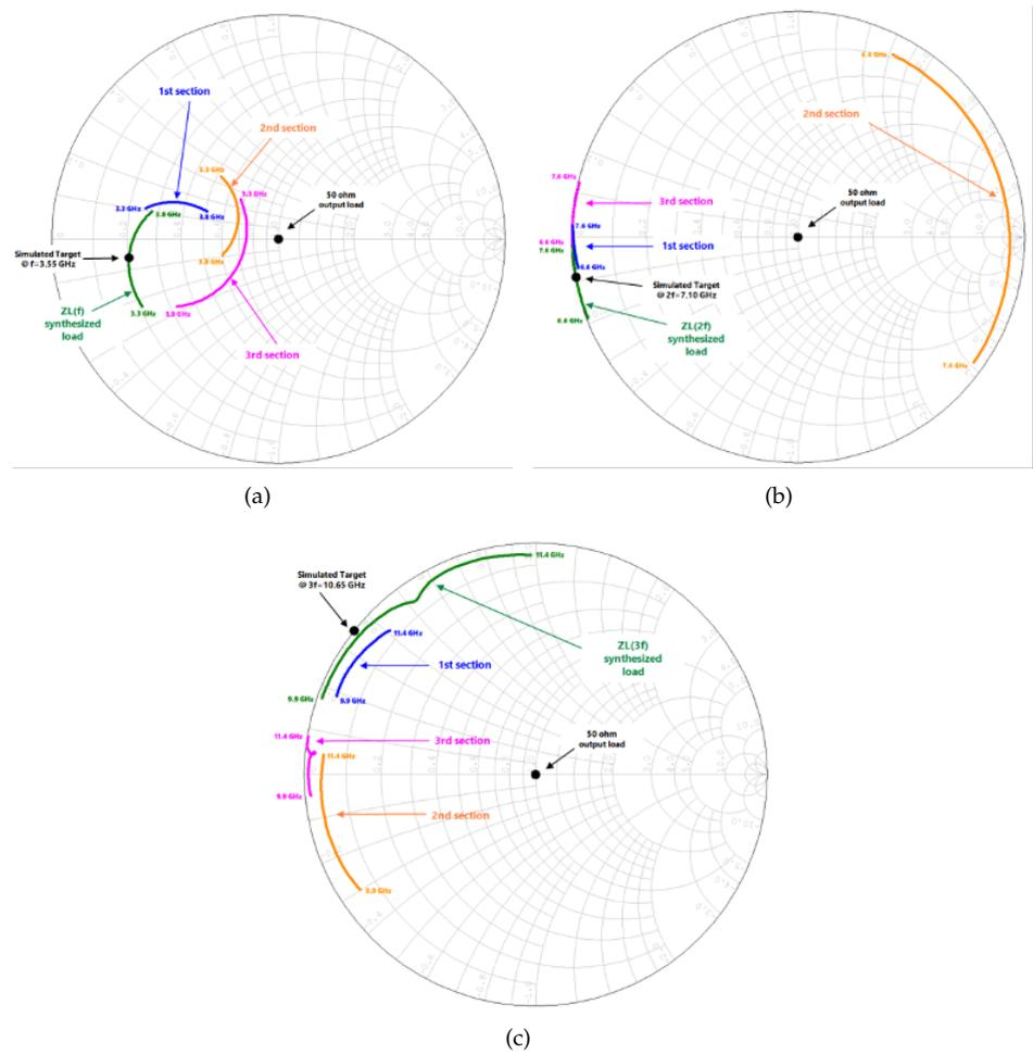
**Figure 8.** Output matching network: synthesized load at the matched port and across each matching network section, for the fundamental frequency (a), the second harmonic (b) and the third harmonic (c), in the frequency range from 3.3 to 3.8 GHz.
