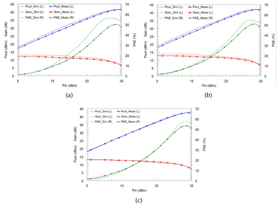
**Figure 16.** Power amplifier performance at 3.4 GHz (a), 3.55 GHz (b) and 3.7 GHz (c).
