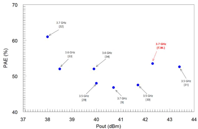
**Figure 19.** State of the art of GaN PA's in graphical form.
