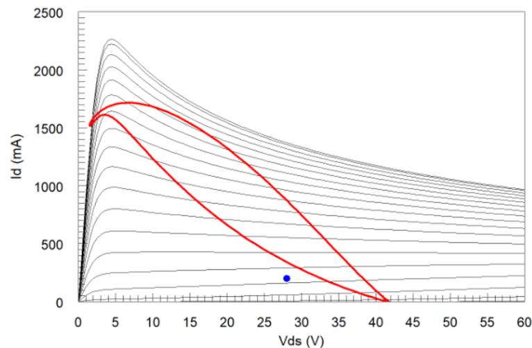
Figure 12. Simulated intrinsic load curve at 1 dBcp.
