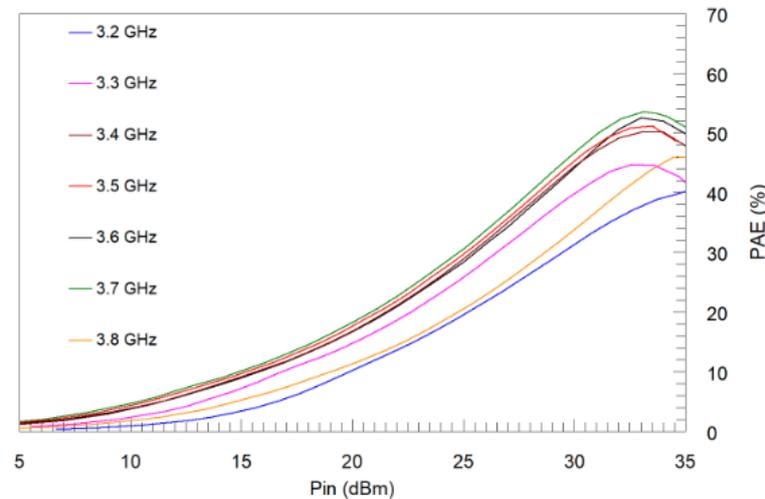
**Figure 17.** Measured PAE values in the frequency range 3.2 GHz - 3.8 GHz.
