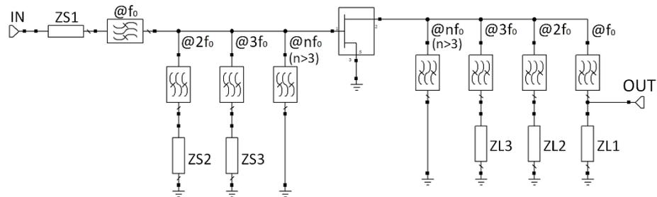
**Figure 1.** Matching networks of an HT PA.
