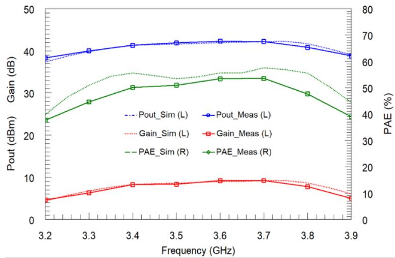
**Figure 18.** PA performance at Pin = 33 dBm.
