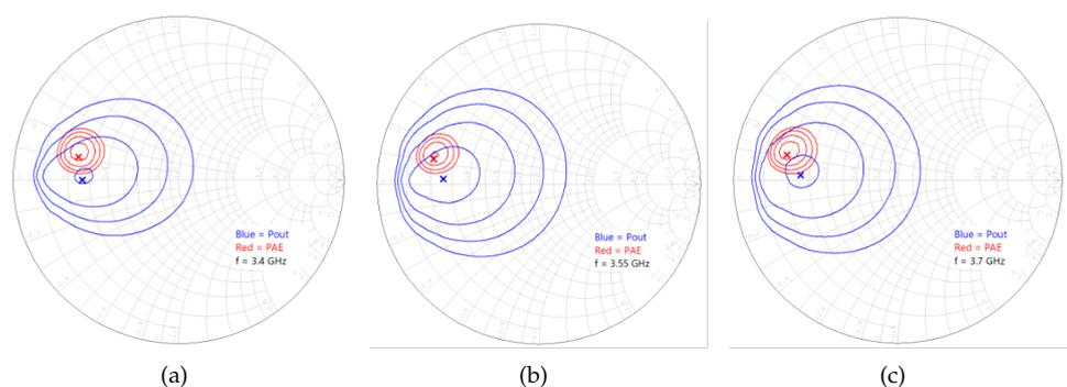
**Figure 4.** Load pull simulations at 3.4 GHz (a), 3.55 GHz (b) and 3.7 GHz (c).
