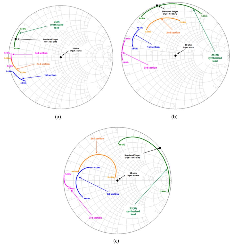
**Figure 10.** Output matching network: synthesized load at the matched port and across each matching network section, for the fundamental frequency (a), the second harmonic (b) and the third harmonic (c), in the frequency range from 3.3 to 3.8 GHz.
