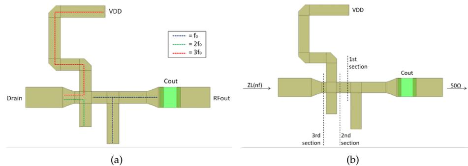
**Figure 7.** Output matching network: transmission line and open stub controlling each harmonic (a) and section planes used to synthesized the whole structure (b).
