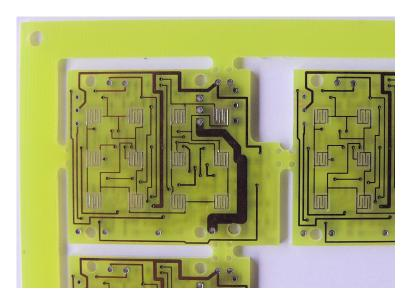
Figure 3. FR4 Printed Circuit Board, showing cut-outs. (JCU Layouts).
