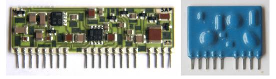
Figure 7. Thick film circuits before and after a protective coating has been applied.
