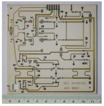
Figure 8. Thick film RF circuit on alumina. (GEC Avionics, designer Kikkert).
