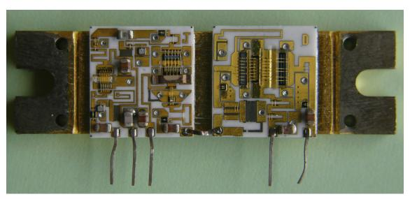
Figure 6. 20 Watt Class C Amplifier Hybrid MHW820 (Motorola).
