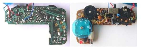
Figure 1 FR3 Printed Circuit Board for a low cost AM / FM radio.
