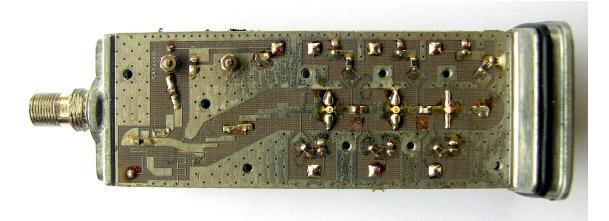
Figure 4. Ku band (12 GHz) Low Noise Converter (LNC) using RF/duroid (Norsat).
