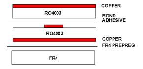
Figure 5. Bonding laminates to form a multilayer board (Courtesy Rogers Corporation).
