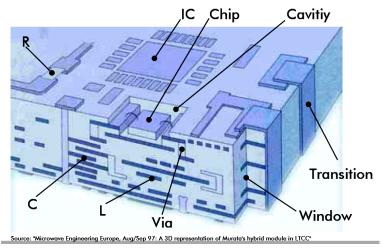
Figure 9. Typical LTCC circuit.
