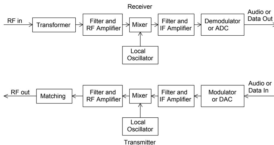
Figure 1. Typical Transmitter and Receiver Block Diagram.
