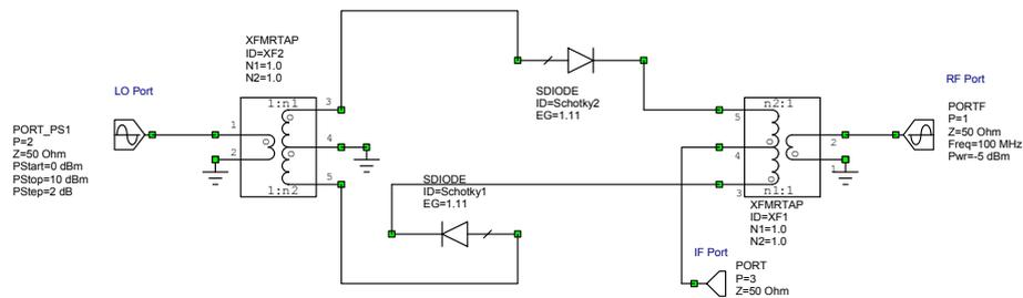
Figure 27 b. Mixer with -ve voltage applied at the IF port.
