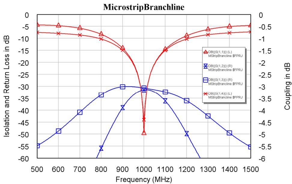
Figure 25. Microstrip Branchline coupler performance.
