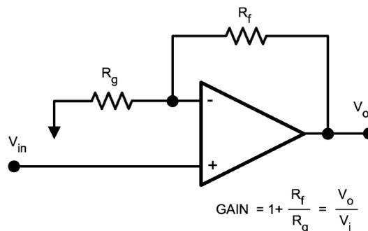
Figure 1. Noninverting Amplifier (National Semiconductor Appl Note OA-30)
