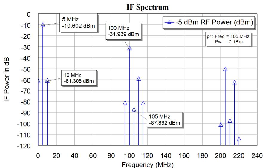
Figure 21. IF spectrum of a balanced diode mixer as a down-converter.
