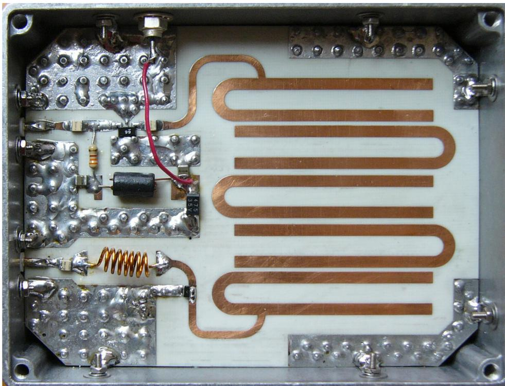
Figure 3. Harmonic Multiplier, to produce 810 MHz from 162 MHz.[1]
