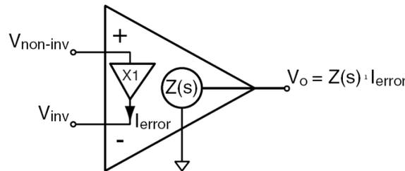
Figure 3 Current Feedback amplifier configuration (National Semiconductor Appl Note OA-30)
