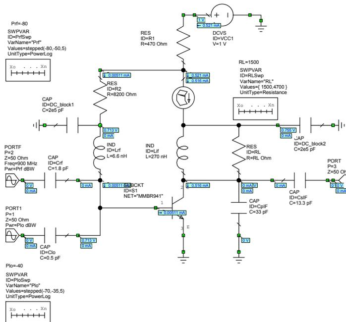
Figure 46. Active single diode mixer (AWR example, Low\_Power\_Mixer).
