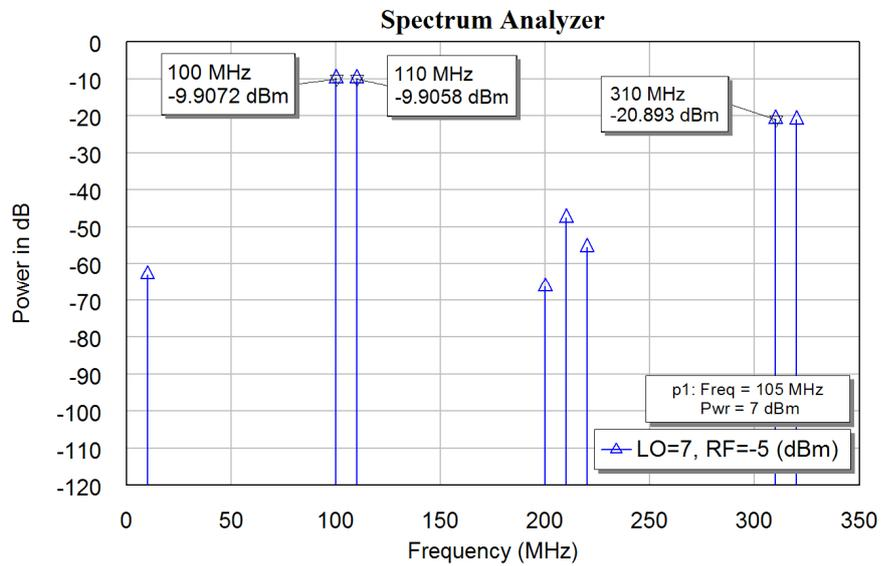
Figure 32. RF spectrum of a double balanced diode mixer as an up-converter.
