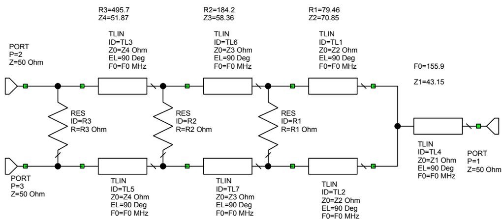
Figure 13. Circuit for a 90 MHz to 270 MHz Wilkinson Hybrid.
