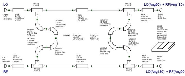
Figure 40. Circuit diagram the Branchline coupler used as a subcircuit in Figure 39.
