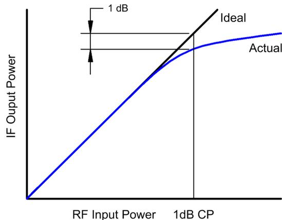
Figure 3. 1 dB Compression Point of a mixer.
