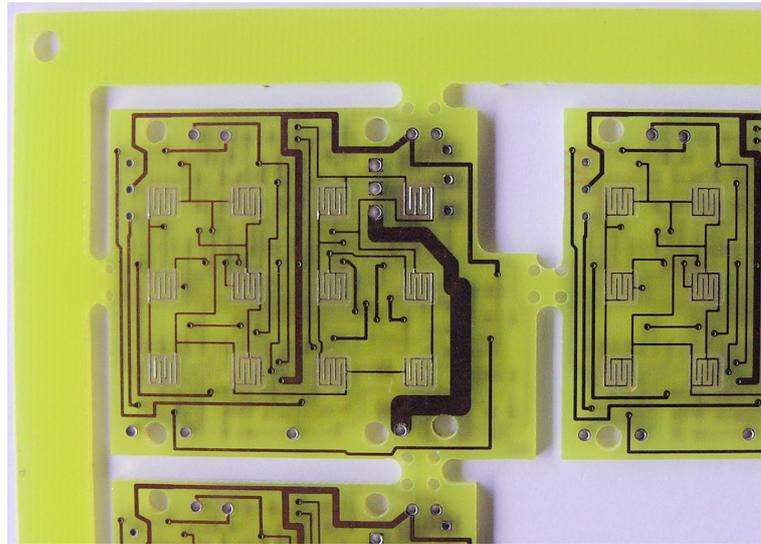
Figure 3. FR4 Printed Circuit Board, showing cut-outs. (JCU Layouts).
