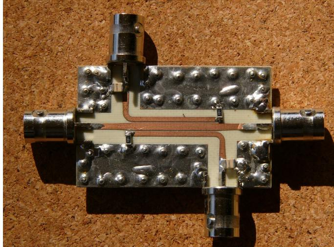
Figure 34. Photograph of the Microstrip-line coupler.
