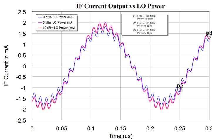
Figure 22. IF currents for a balanced diode mixer as a down-converter.
