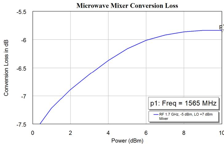
Figure 37. Conversion loss of a Microwave Balanced Diode mixer.
