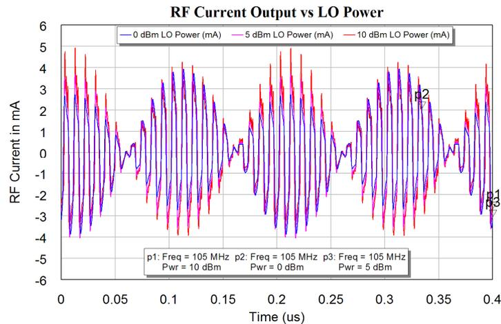
Figure 24. RF currents for a balanced diode mixer as an up-converter.
