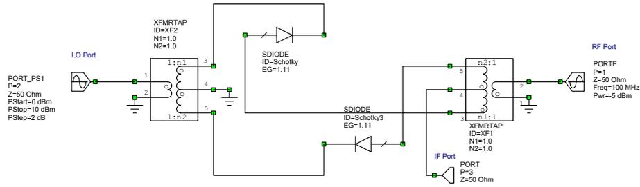
Figure 27a Mixer with +ve voltage applied at the IF port.
