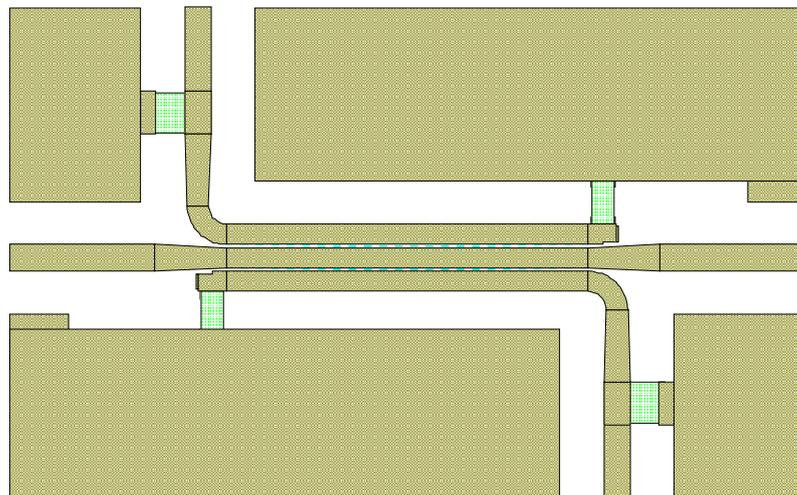
Figure 33. Layout of Microstrip-line coupler.
