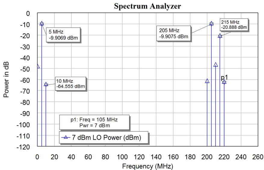
Figure 29. IF spectrum of a double balanced diode mixer as a down-converter.
