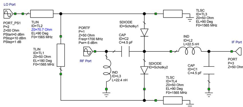
Figure 36. Circuit diagram of a Microwave Balanced mixer.
