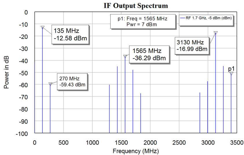
Figure 43. IF spectrum of a balanced mixer with a Branchline coupler.
