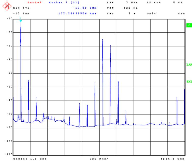
Figure. 45, Measured spectrum of Branchline coupler mixer of figure 44.
