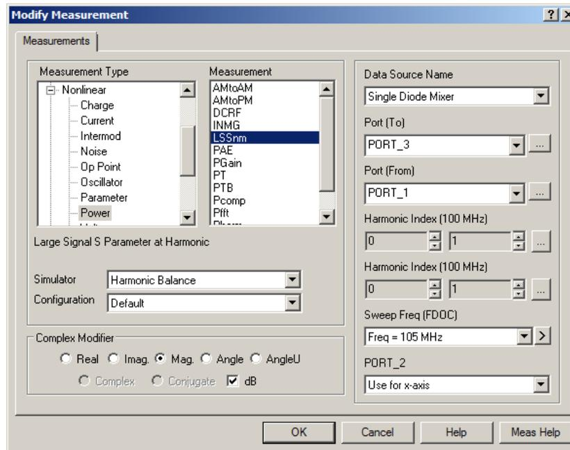
Figure 10. Parameters for conversion loss measurements.
