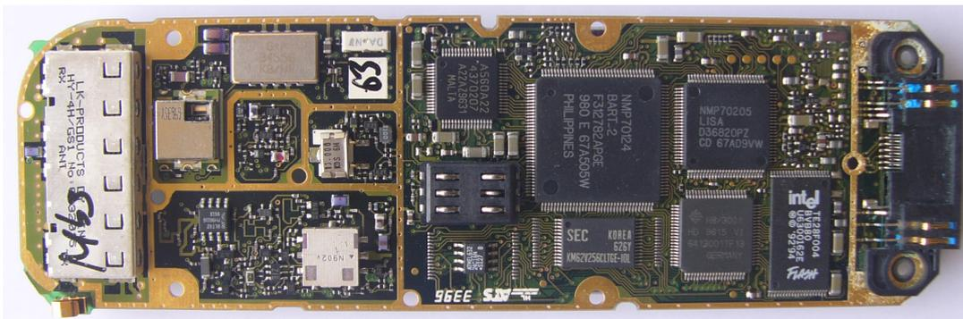
Figure 2. FR4 Multilayer Printed Circuit Board. (Nokia Mobile Phone).
