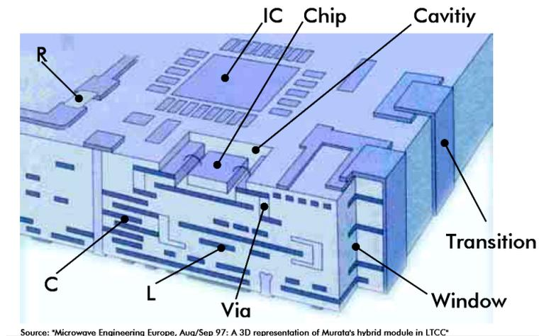
Figure 9. Typical LTCC circuit.
