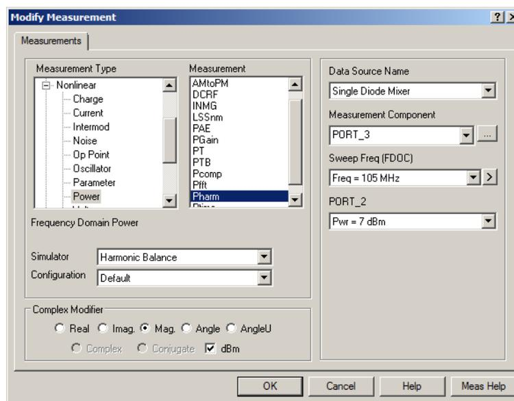
Figure 12. Frequency domain power measurement.
