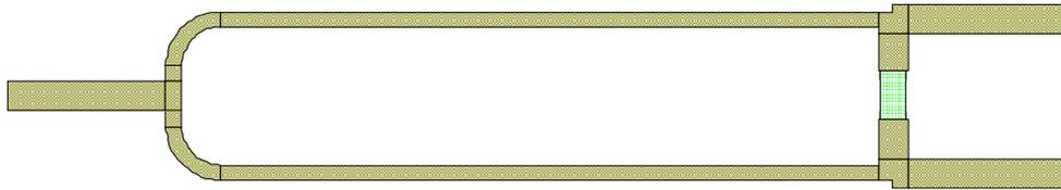
Figure 7. PCB layout of a Wilkinson Hybrid.
