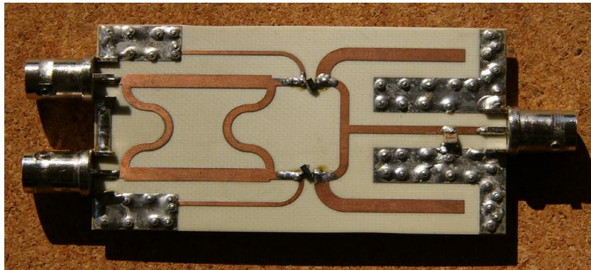
Figure 44. Hardware realisation of the balanced mixer using a Branchline coupler.
