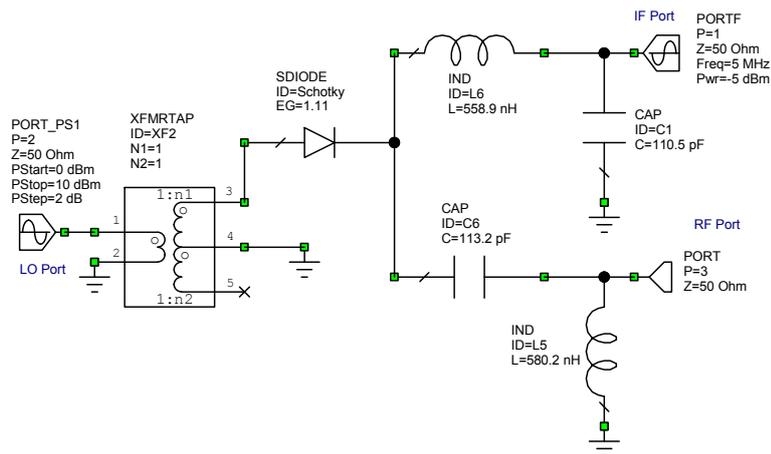
Figure 16. Circuit diagram of a single diode mixer as an up-converter.
