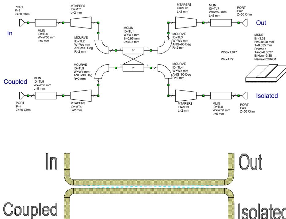
Figure 30.  $\lambda/4$  20 dB coupler Schematic and Corresponding Microstrip Layout.
