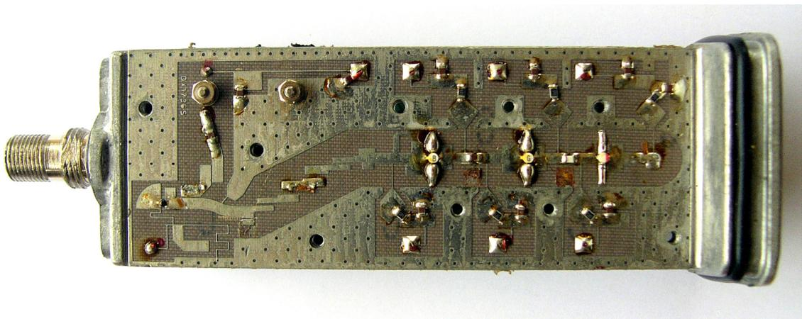
Figure 4. Ku band (12 GHz) Low Noise Converter (LNC) using RF/duroid (Norsat).
