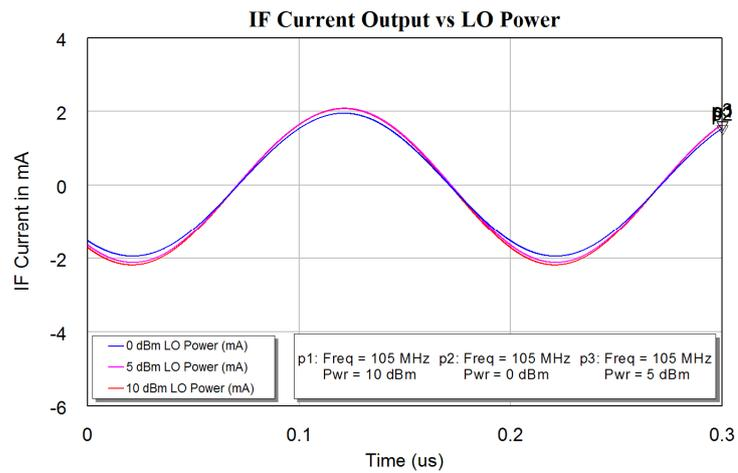
Figure 31. IF currents of figure 29 with frequency components >25 MHz removed.
