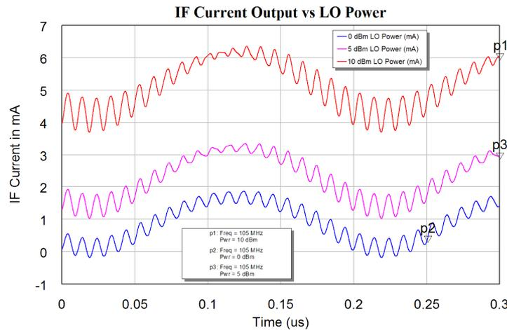
Figure 15. IF currents for a single diode mixer as a down-converter.
