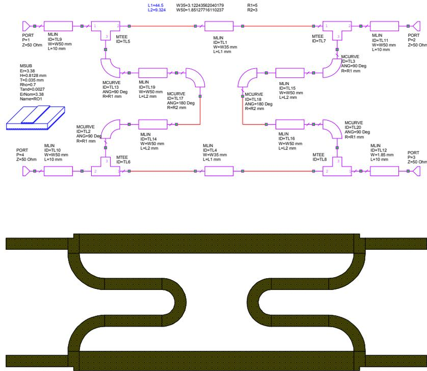
Figure 24. Branchline coupler Schematic and corresponding PCB layout.
