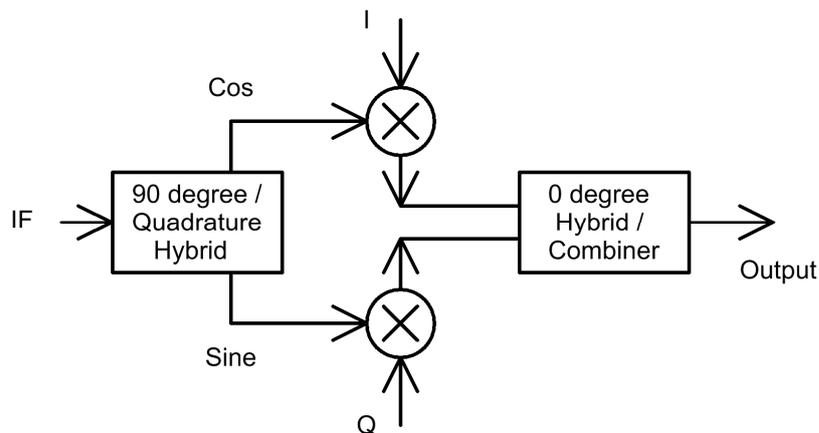
Figure 54. Block diagram of a quadrature mixer.
