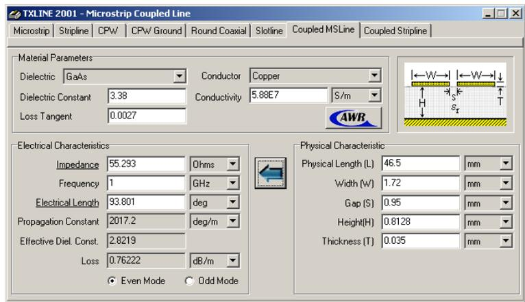
Figure 29. Calculated geometry for a  $\lambda/4$  20 dB coupler.
