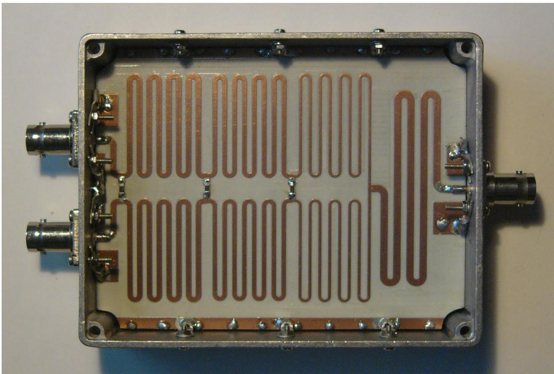
Figure 14. Hardware for 90 MHz to 270 MHz Wilkinson Transmission-line Hybrid.
