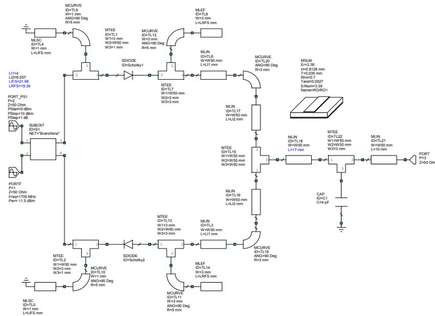
Figure 39. Circuit diagram of a balanced mixer with a Branchline coupler.
