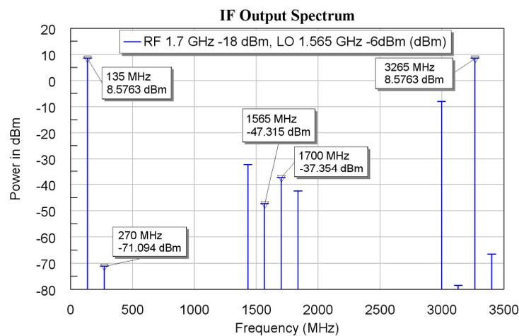
Figure 49. IF spectrum of the Gilbert Cell mixer of figure 45 as a down-converter.
