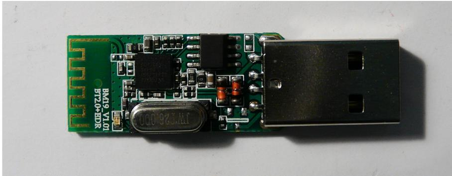
Figure 2. Typical Consumer RF Module. (Unbranded EDR Bluetooth USB Adapter)
