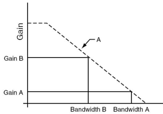
Figure 2. Open loop and Closed loop gain of Voltage Feedback Amplifier (National Semiconductor Appl Note OA-30)
