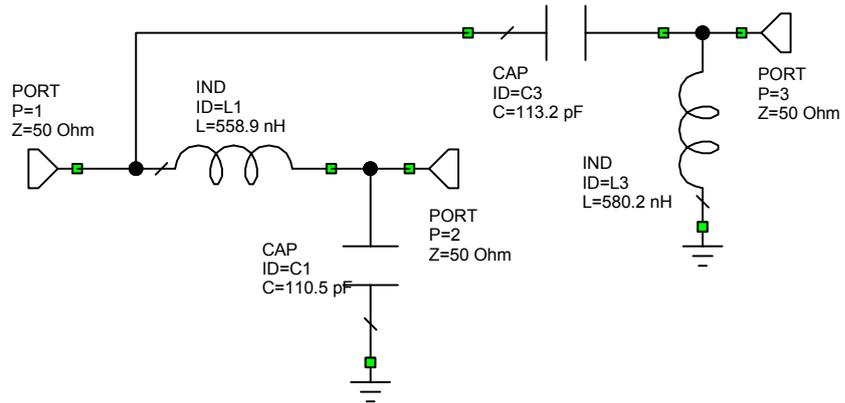
Figure 6. Diplexer circuit.
