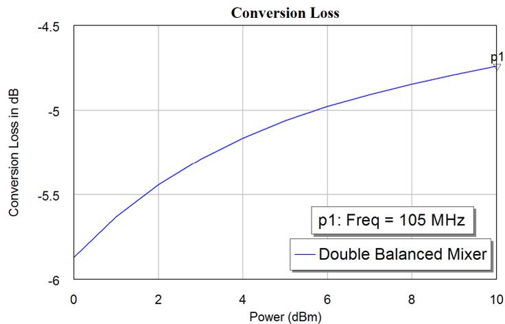
Figure 28. Conversion loss of a double balanced diode mixer.
