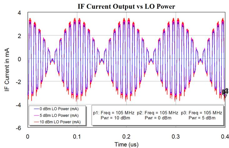
Figure 33. RF currents for a double Balanced Diode Mixer as an up-converter.
