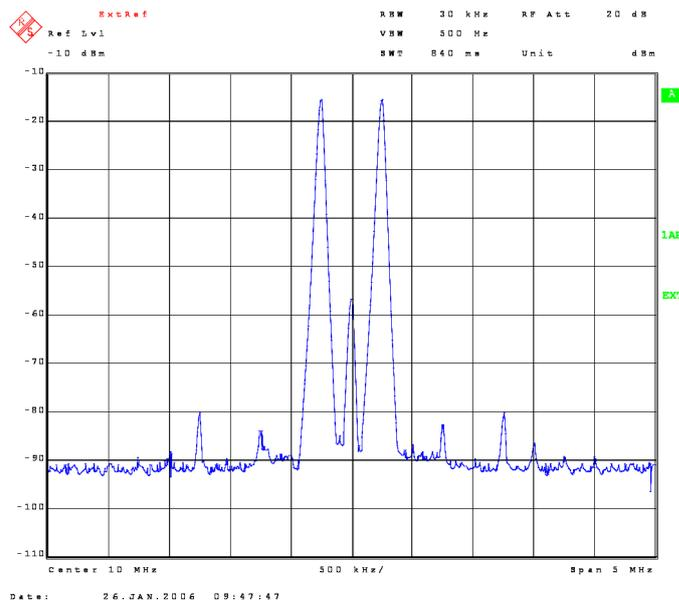
Figure 35. Measured performance of the mixer of figure 34.
