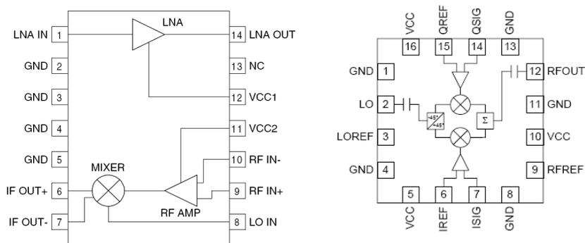
Fig 52. RF MicroDevices RF2411 LNA and Mixer and RF2850, IQ active mixer
