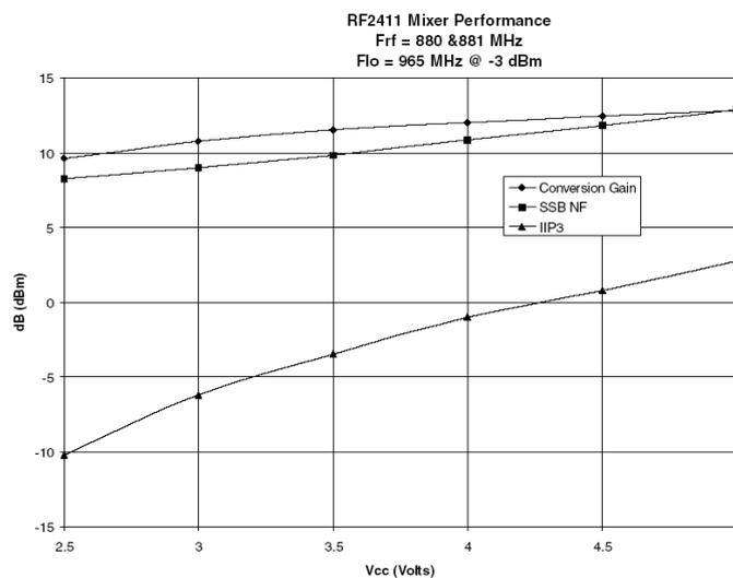
Figure 53. RF MicroDevices RF2411 LNA and mixer performance.
