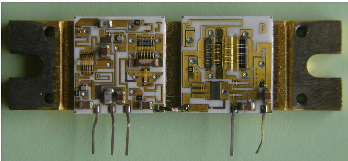
Figure 6. 20 Watt Class C Amplifier Hybrid MHW820 (Motorola).
