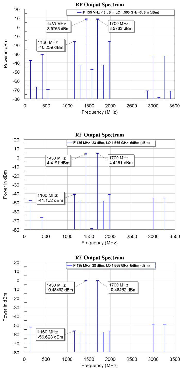
Figure 50. RF spectra of the Gilbert Cell mixer of figure 47 as an up-converter, RF levels of -18dBm (top), -23 dBm (middle) -28 dBm (bottom).
