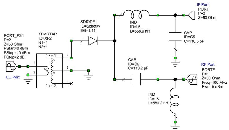
Figure 8. Circuit diagram of a single diode mixer as a down-converter.
