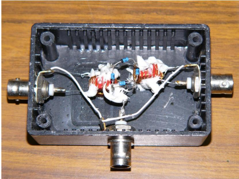
Figure 34. Construction of a Double Balanced Mixer for use in Practical Sessions.
