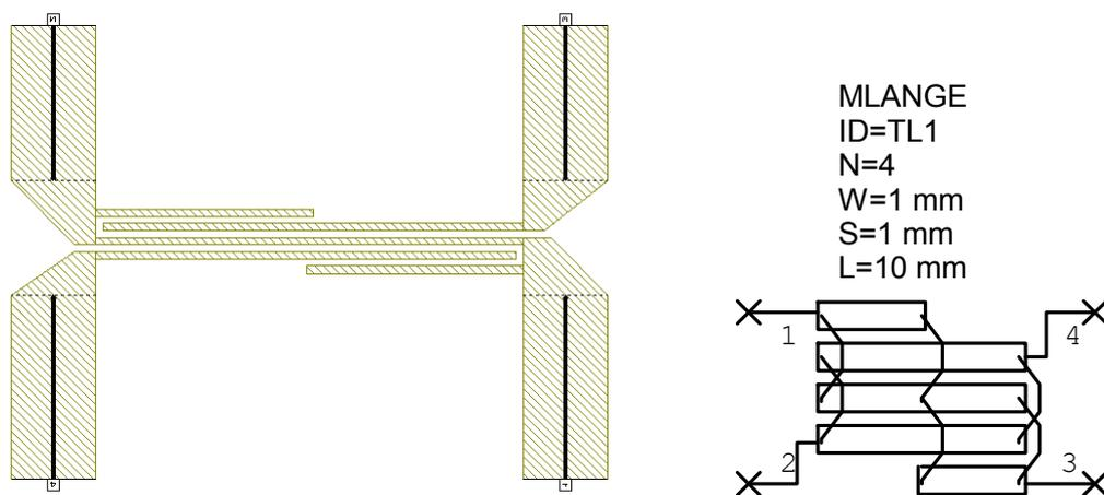
Figure 36. Lange coupler layout (the bond wires are not shown) and schematic.
