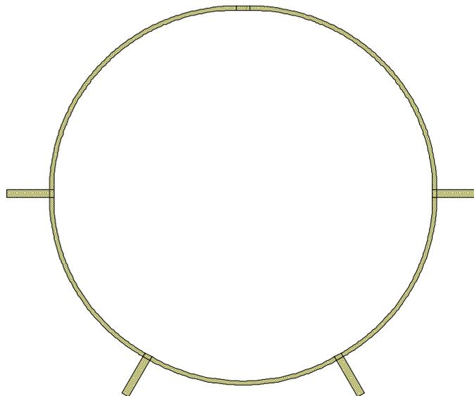
Figure 19. PCB layout of a  $1.5 \lambda$  Rat-race Hybrid
