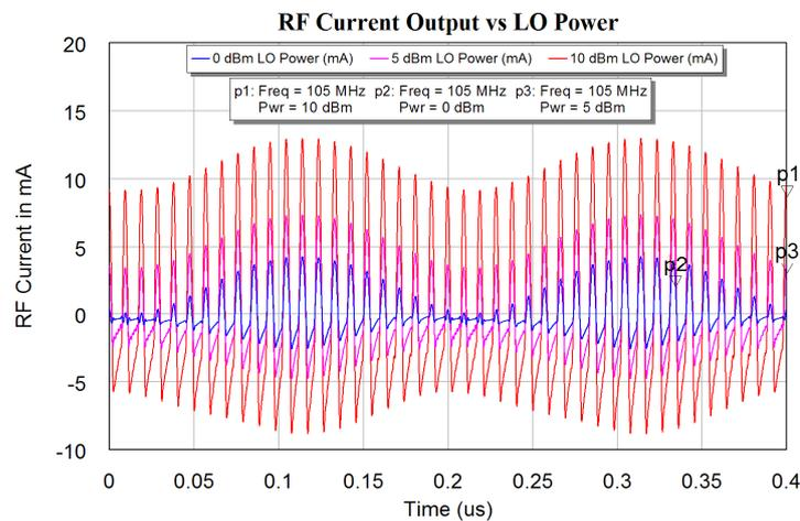
Figure 18. RF currents for a single diode mixer as an up-converter.
