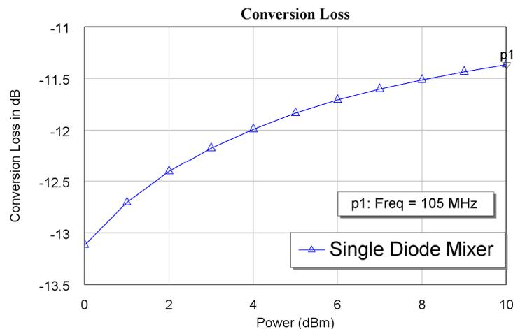
Figure 11. Conversion loss of a single diode mixer.
