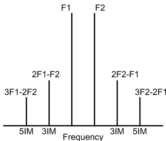
Figure 4. IM distortion of an amplifier or mixer.
