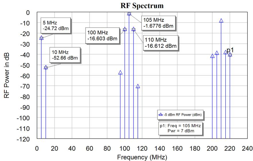
Figure 17. RF spectrum of a single diode mixer as an up-converter.
