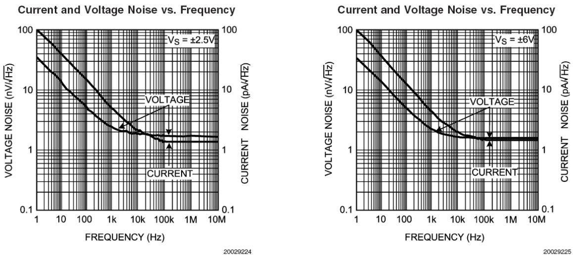
Figure 6. Noise of LMH6622 versus frequency
