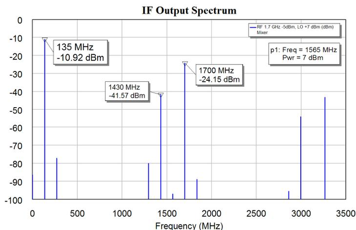
Figure 38. IF Spectrum of a Microwave Balanced Diode mixer as a down-converter.
