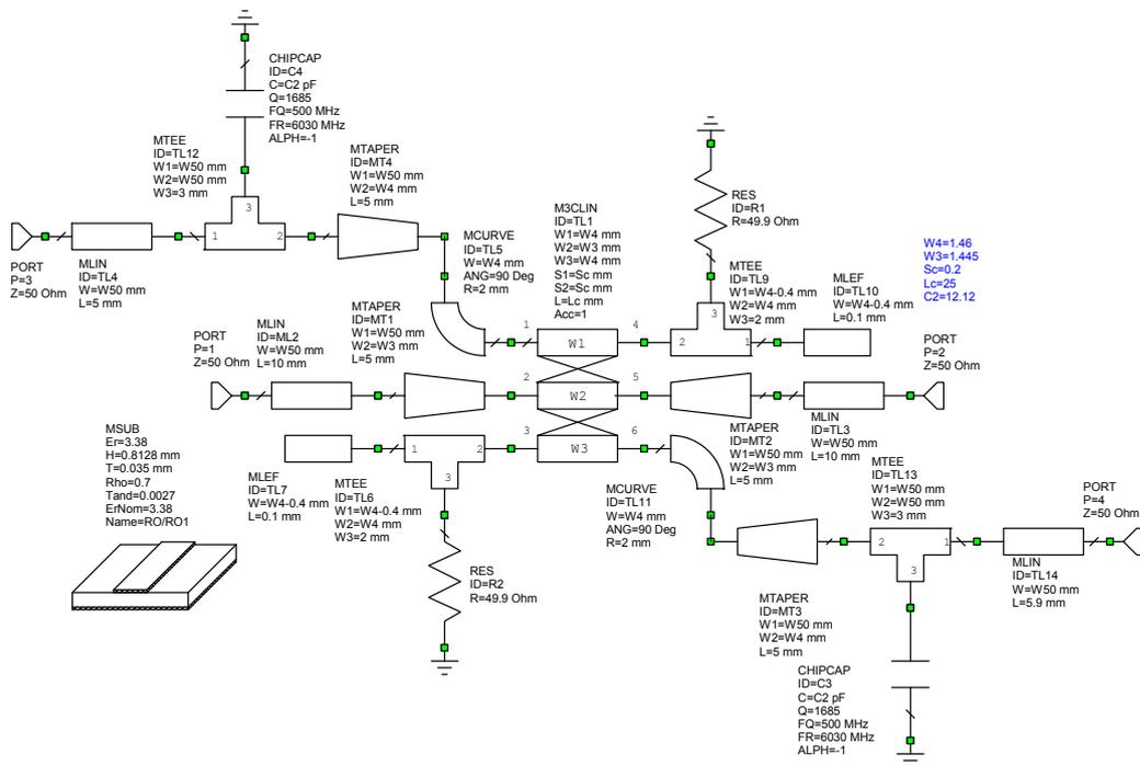
Figure 35. Circuit diagram of Microstrip-line coupler.
