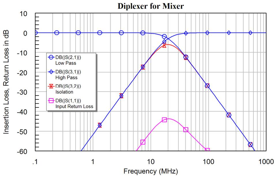
Figure 7. Frequency response of diplexer after optimisation.
