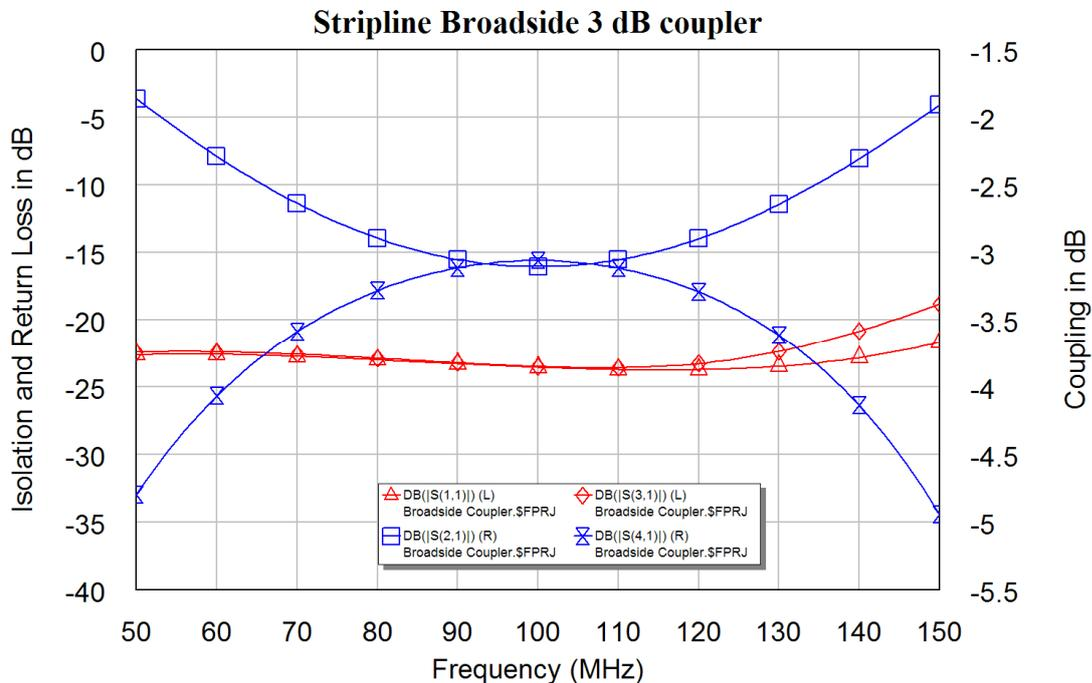
Figure 41. Performance of broadside coupled-line circuit using SBCPL element.
