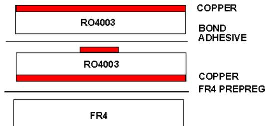
Figure 5. Bonding laminates to form a multilayer board (Courtesy Rogers Corporation).
