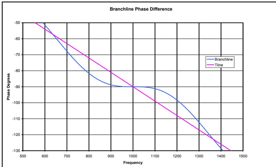
Figure 26. Branchline coupler phase difference between output ports.
