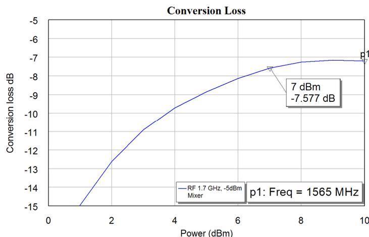
Figure 42. Conversion loss of a balanced mixer with a Branchline coupler.
