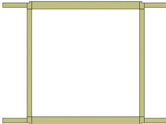
Figure 21. Branchline coupler PCB layout.
