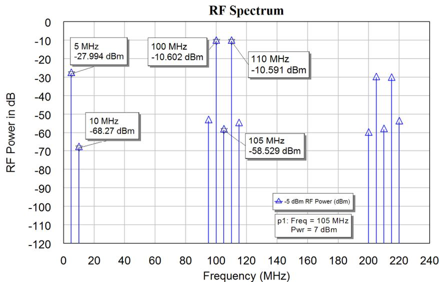
Figure 23. RF spectrum of a balanced diode mixer as an up-converter.
