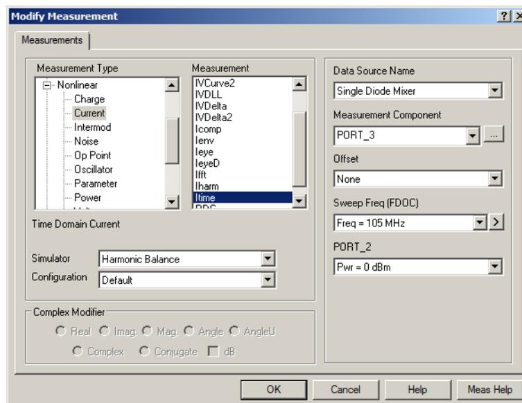
Figure 14. Itime measurement setting.
