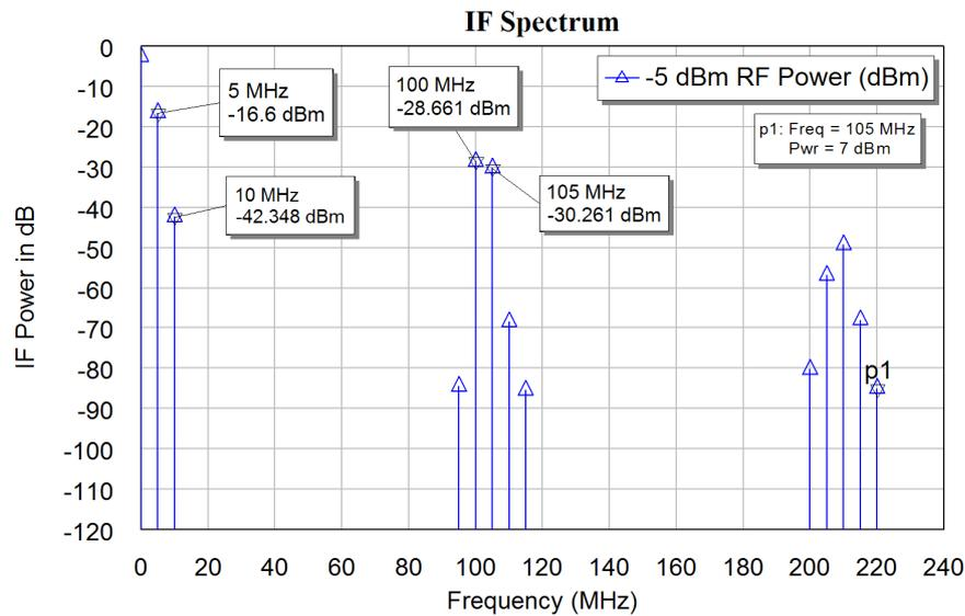
Figure 13. IF spectrum of a single diode mixer as a down-converter.
