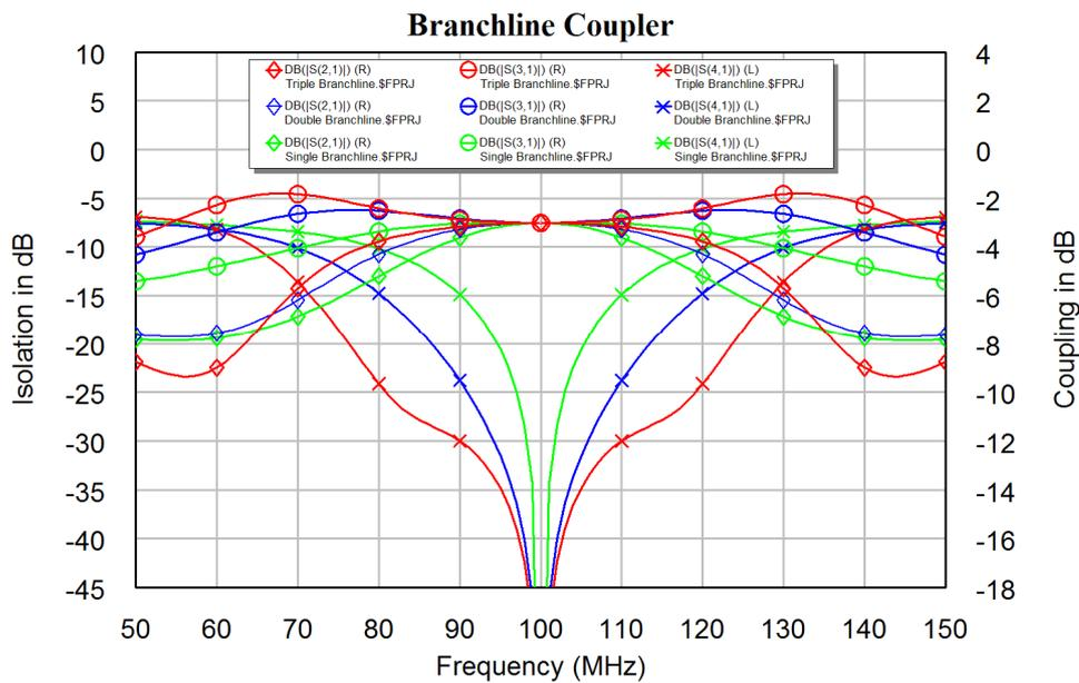
Figure 28. Multi-loop Quadrature Hybrid performance.
