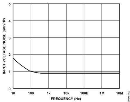
Figure 2. AD797 Voltage Noise Spectral Density
