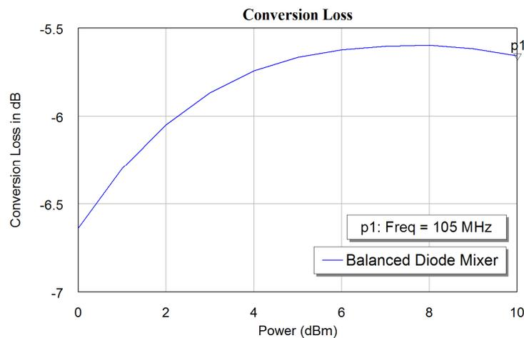
Figure 20. Conversion loss of a balanced diode mixer.
