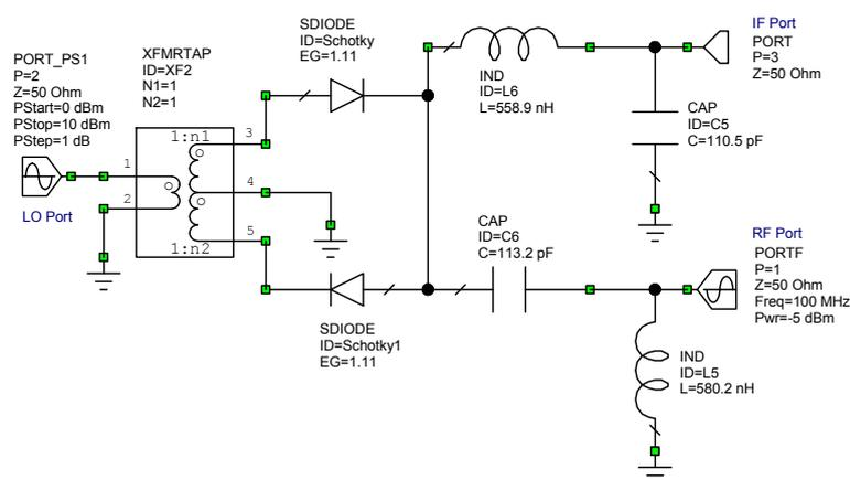
Figure 19. Circuit diagram of a balanced mixer.
