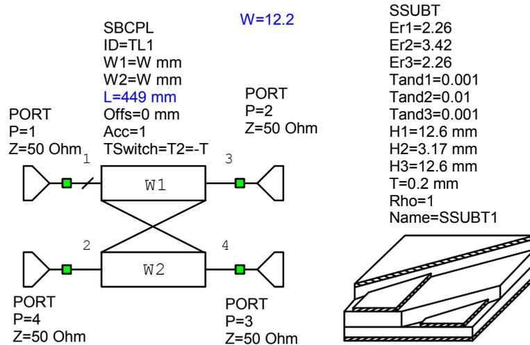
Figure 40. MWO broadside coupled-line circuit using SBCPL.
