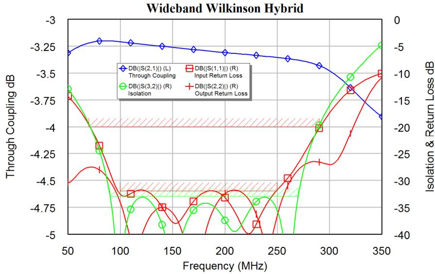
Figure 15. Simulated performance of the Hybrid of figure 14.
