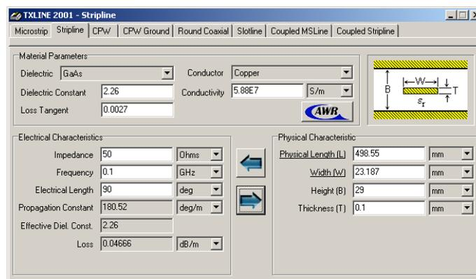
Figure 39. Terminating line-width calculation.
