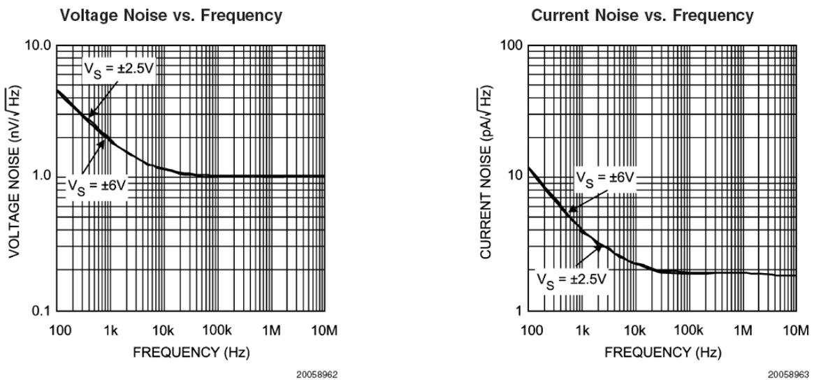
Figure 5. Noise of LMH6624L versus frequency
