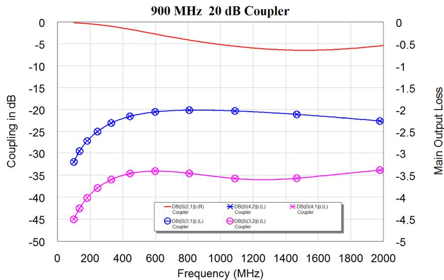
Figure 32. Simulated performance of stripline coupler.
