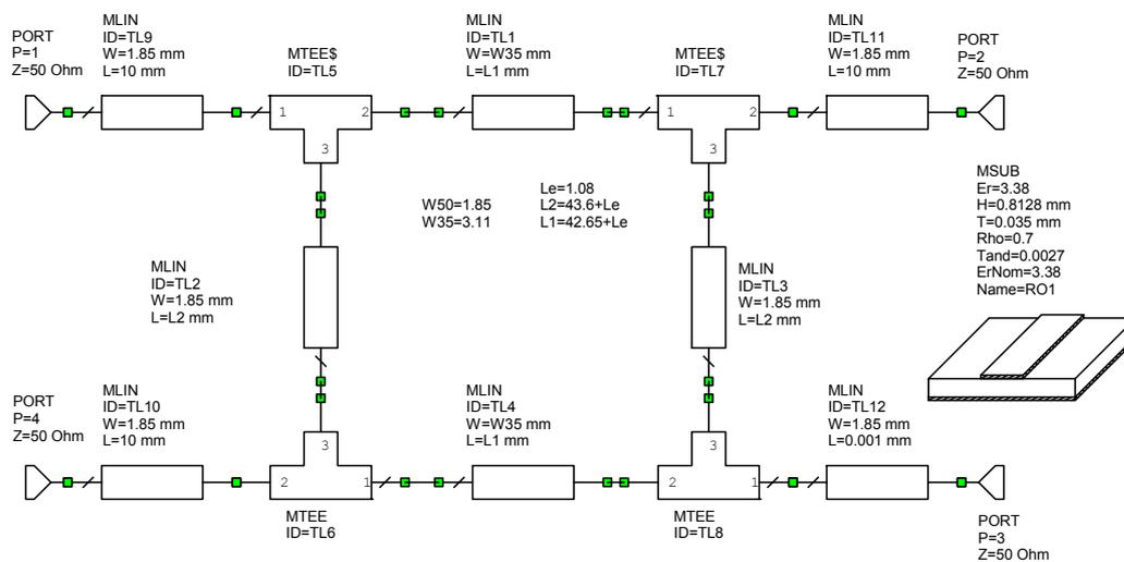
Figure 20. Branchline coupler circuit
