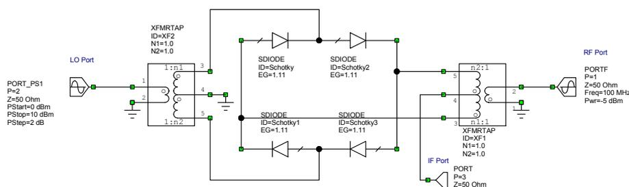
Figure 26. Circuit diagram of a double balanced mixer.
