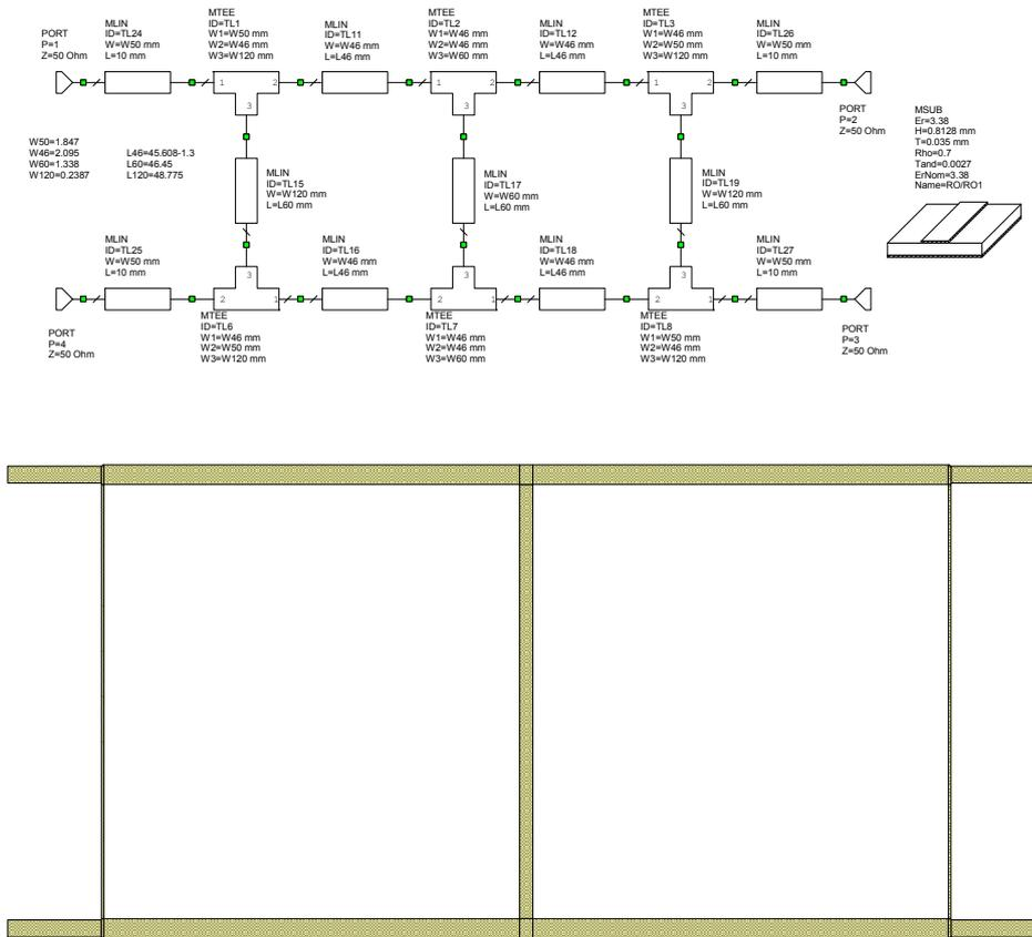
Figure 27. Wideband Quadrature Hybrid Schematic and the corresponding PCB layout.
