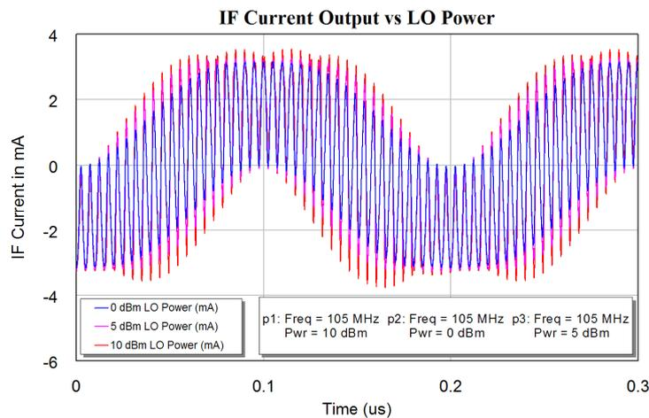
Figure 30. IF currents for a balanced diode mixer as a down-converter.
