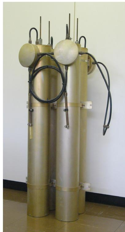
Figure 78. Coaxial cavity diplexer for 80 MHz.
