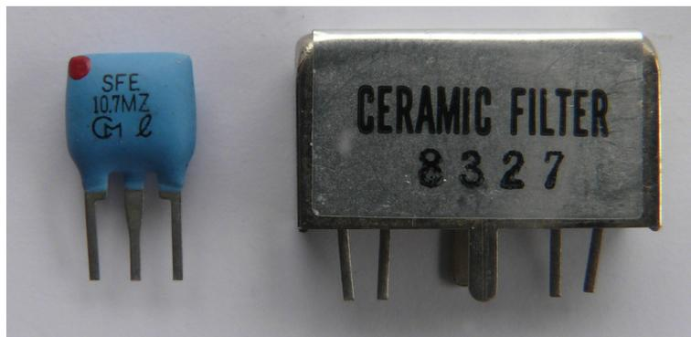
Figure 73. 10.7MHz ceramic IF filters.
