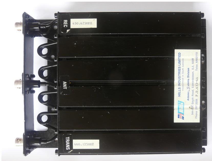
Figure 80. Cavity filter diplexer for mobile radio applications.
