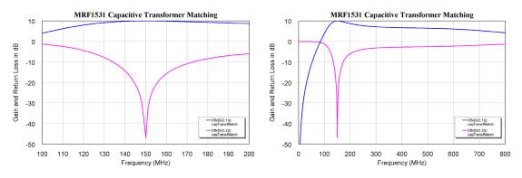
Figure 18. Frequency Response of the Bandpass L Matching Network.
