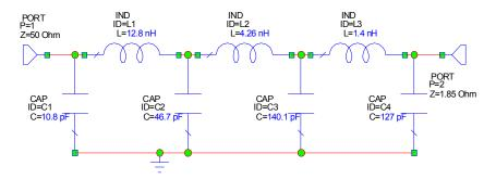
Figure 25. Starting Broadband Match Schematic
