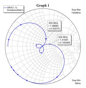
Figure 30. Final Broadband Match Input Impedance.
