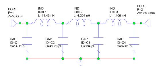
Figure 28. Final Broadband Match Schematic
