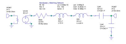
Figure 15. Circuit representation of the input impedance and the matching network.
