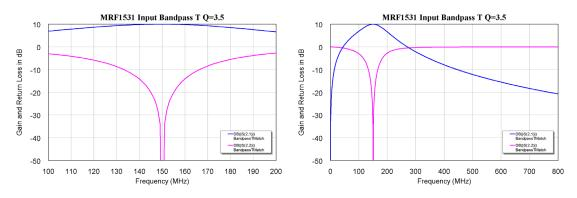
Figure 14. Frequency Response of the Bandpass T Matching Network (Harmonic View)
