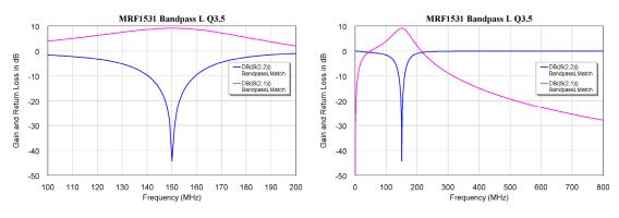
Figure 16. Frequency Response of the Bandpass L Matching Network
