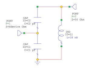
Figure 5. Capacitive Impedance Transformer Matching Network.
