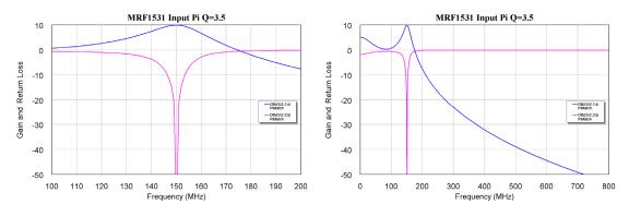
Figure 10. Frequency Response of the Pi Matching Network
