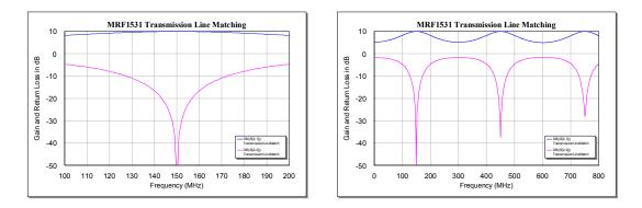
Figure 23. Frequency Response of the Transformer Match.
