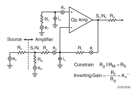
Figure 4 Noise sources in an operational amplifier configuration (National Semiconductor Appl Note OA-11)
