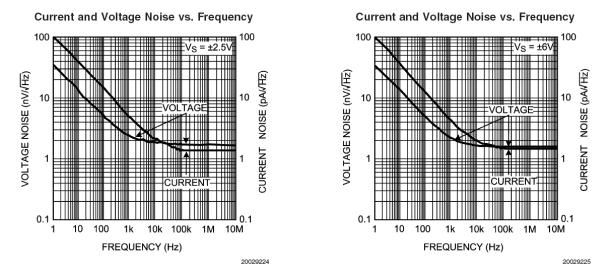
Figure 6. Noise of LMH6622 versus frequency
