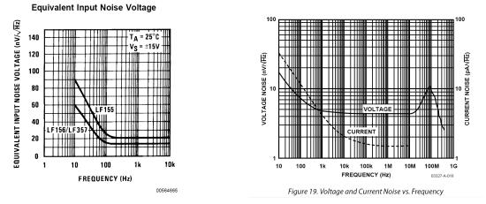
Figure 7. Noise of LF356 and AD8027/AD8028 versus frequency
