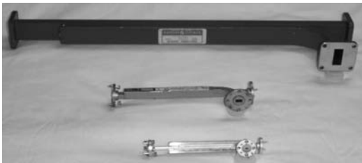
Figure E-16 Directional coupler in rectangular waveguide: (a) schematic of a directional coupler; (b) waveguide directional coupler showing coupling slots; and (c) and (d) photograph of three directional couplers with the fourth port terminated in an integral matched load. In (c) and (d), from top-to-bottom, W-band and 10 cm long, Ka-band and 15 cm long, and X-band 35 cm long.
