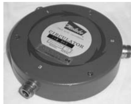
Figure 7-33 A coaxial circulator showing three ports and the direction of circulation. The ferrite disc is located in the center of the circulator and is topped by an enclosed permanent magnet.
