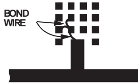
Figure 4-20 Open-circuited stub with variable length realized using wire bonding from the fixed stub to one of the bond pads.
