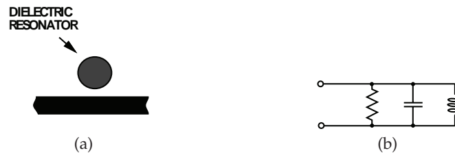
Figure 7-31 Dielectric resonator: (a) microstrip transmission line with a coupled dielectric resonator; and (b) parallel RLC resonant circuit.
