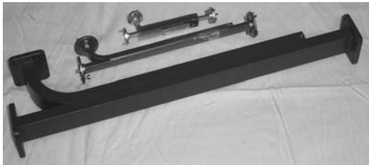
Figure E-16 Directional coupler in rectangular waveguide: (a) schematic of a directional coupler; (b) waveguide directional coupler showing coupling slots; and (c) and (d) photograph of three directional couplers with the fourth port terminated in an integral matched load. In (c) and (d), from top-to-bottom, W-band and 10 cm long, Ka-band and 15 cm long, and X-band 35 cm long.
