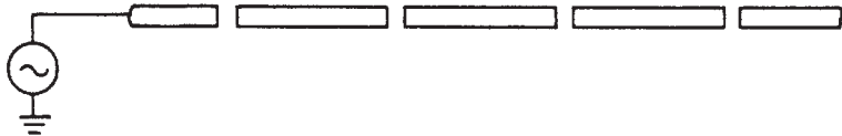
Figure 10-84 General microstrip layout for an end-coupled bandpass filter (series coupling gaps between cascaded straight resonator elements).
