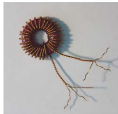
Figure 5. A trifilar wound RF Transformer
