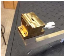
The cavity was tested using an **Agilent E8363C Precision Network Analyzer (PNA)**
