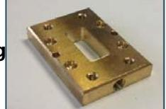
The **cavity was manufactured** in the mechanical workshop of the ISS, by mechanical specialists, using **pure brass** (instead of silver).
