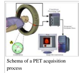
Schematic view of a detector block and ring of a PET scanner
