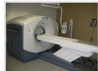
PET/CT-System with 16-slice CT; the ceiling mounted device is an injection pump for CT contrast agent
