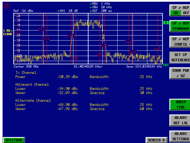
Fig. 2-1 Measuring the relative adjacent channel power of an NADC signal in each of the two adjacent channels below and above the transmit channel.
